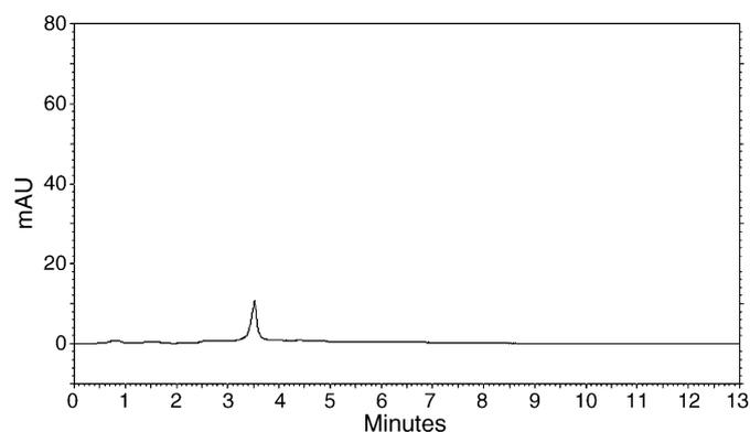
Fig. 5. Chromatogram of placebo sample in borate buffer pH 9.0. Chromatographic conditions: Hypersil Keystone Betabasic C8 (250 mm  $\times$  4.6 mm; 5  $\mu\text{m}$ ); mobile phase acetonitrile–water (35:65, v/v); flow rate  $1.0 \text{ ml min}^{-1}$ ; injection volume  $20.0 \mu\text{l}$ ; detection UV 282 nm and temperature of  $30 \pm 1^\circ\text{C}$ .
