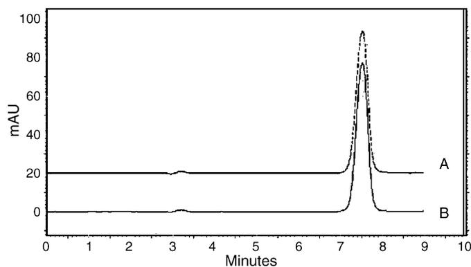
Fig. 4. Chromatograms of rabeprazole sodium (A) reference standard; (B) commercial sample (both at  $40 \mu\text{g ml}^{-1}$ ). Chromatographic conditions: Hypersil Keystone Betabasic C8 (250 mm  $\times$  4.6 mm; 5  $\mu\text{m}$ ); mobile phase acetonitrile–water (35:65, v/v); flow rate  $1.0 \text{ ml min}^{-1}$ ; injection volume  $20.0 \mu\text{l}$ ; detection UV 282 nm and temperature of  $30 \pm 1^\circ\text{C}$ .
